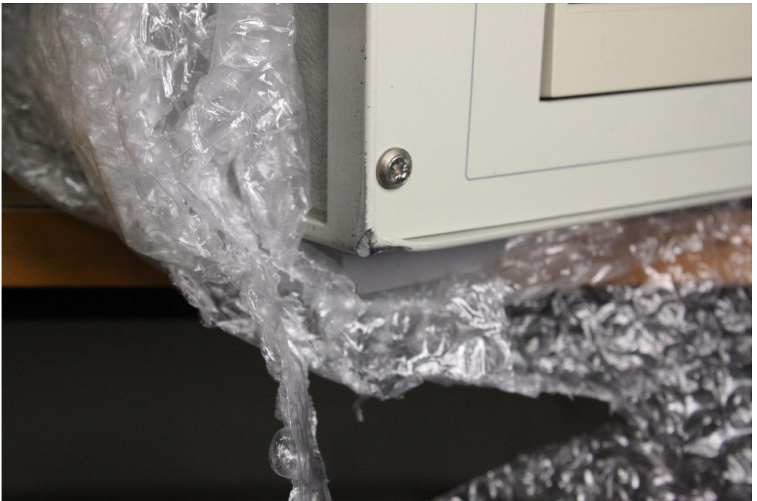
ANOTHER bad impact damage to the front frame. This one to the lower left corner.
