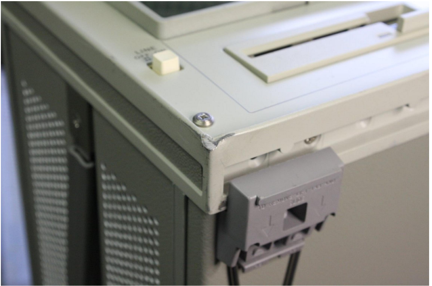
Box cardboard penetration from the lower left ding.
