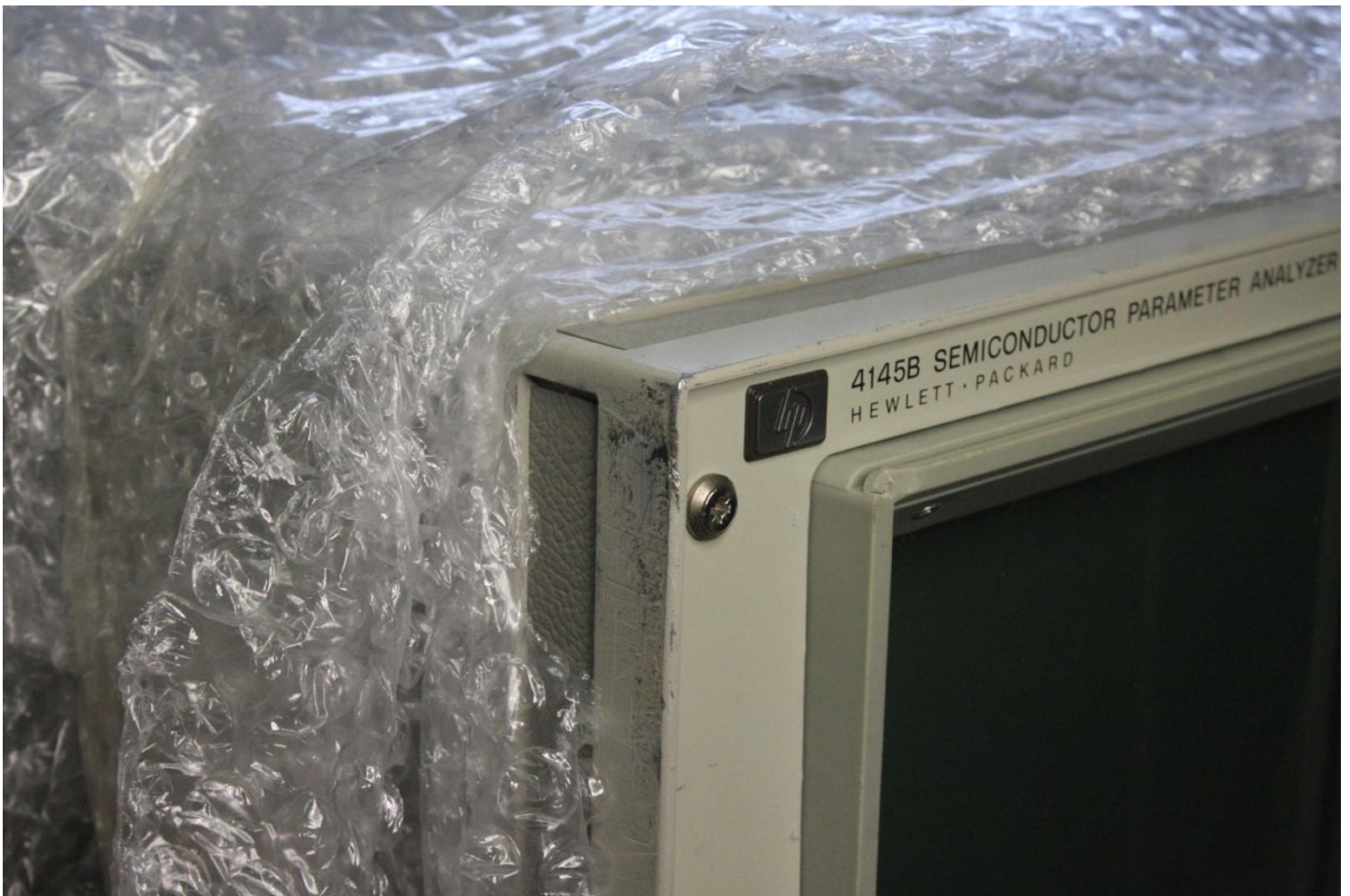
ANOTHER bad impact damage to the front frame. This one to the lower left corner.
